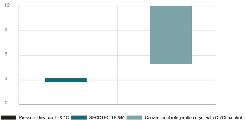
refrigeration dryers, on the other hand, ensure material-friendly operation thanks to their high thermal storage capacity. Once the thermal mass has been charged, the refrigerant compressor and fan motor can remain switched off for much longer without impacting pressure dew point stability.
